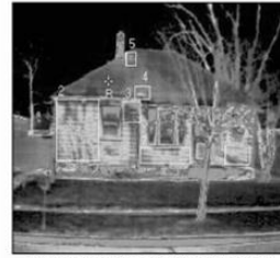
Home above shows heat loss throughout the exterior walls. Details: 800 square foot ranch Exterior walls: Wood and typical insulation Average heat bill $200/month
