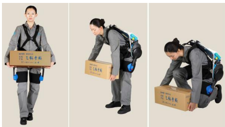
Figure 2. Exoskeleton AWN-03 developed by Panasonic and Activelink to provide lower back support for workers.
